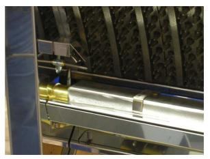
•Remove all spark gas and clean the grill it with a cloth soaked in rubbing alcohol.
