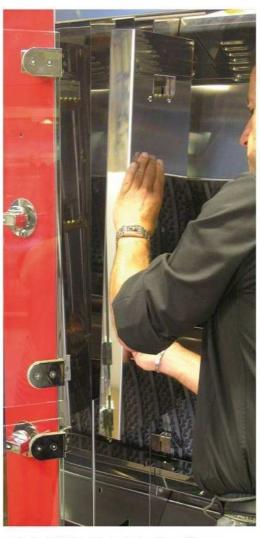
• On the one hand raise the double-wall superior way to match the large diameter of the buttonholes with the screw heads located in the recess of the interior panels and then remove it.
