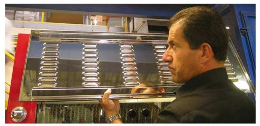
• Take the deflector so that the two stiffeners are directed upward and open vents to the rear.
