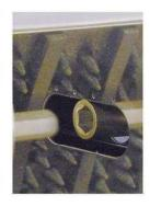
• Introduce the hex end motor located in the nozzle right side of the rotisserie
