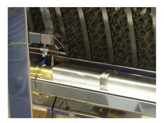
•Loosen the two M4 screws with a wrench, pipe or eye of 7 and remove.
